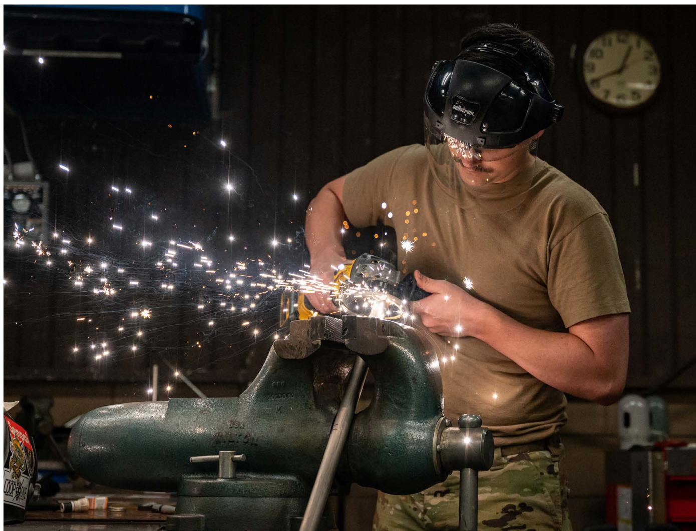
Staff Sgt. Gregory Bailey, 51 st Maintenance Squadron metals technician, operates an angle grinder at Osan Air Base, South Korea. In the event of an aircraft component breaking, the 51 st MXS aircraft metals technology section is tasked with repairing it or fabricating a new component from scratch, ensuring the swift and efficient continuation of aircraft operations.
