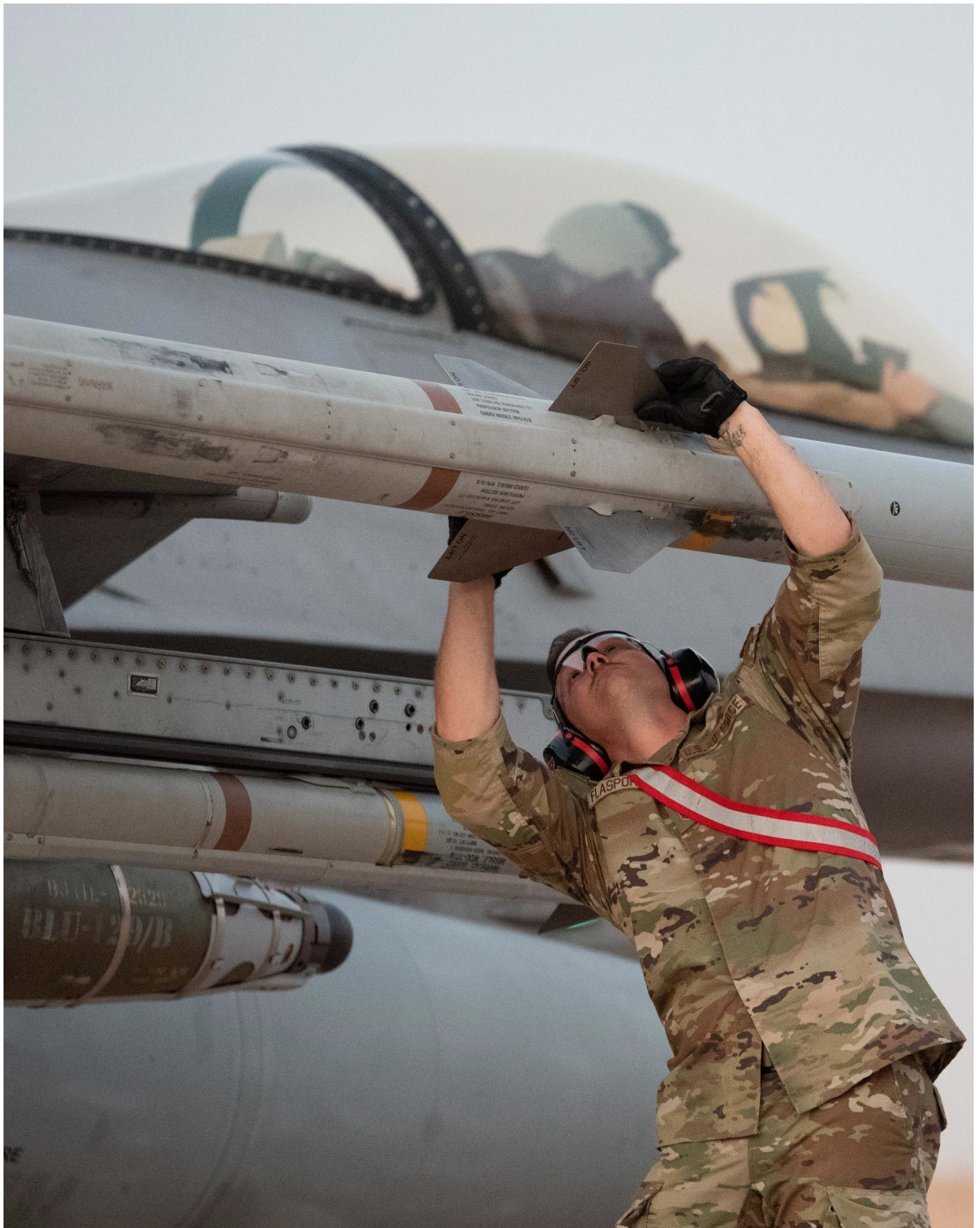
USAF Master Sgt. Dustin Flaspohler, 138 th Fighter Wing aircraft armament systems specialist, performs weapons checks on an F-16 Fighting Falcon assigned to the 125 th Expeditionary Fighter Squadron, after hot pit refueling at Prince Sultan Air Base, Saudi Arabia. Hot pit refueling occurs after an aircraft has landed and is still running its engine allowing for refueling in austere locations. —Photo: USAF photo by Tech. Sgt. Alexander Frank
