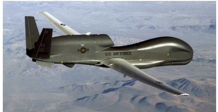
An RQ-4 Global Hawk soars through the sky to record intelligence, surveillance, and reconnaissance data. Air Force and Navy officials met to discuss joint training with the RQ-1. (Courtesy photo by USAF)
