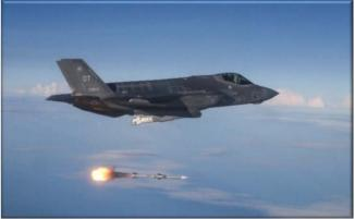
F-35A Lightning II test aircraft releases a AIM-120 missile at targets during live-fire tests over the Joint Gulf Range Complex
