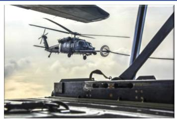
A HH-60G Pavehawk I helicopter receives fuel from an HC-130J Combat King II aircraft during an aerial refueling mission
