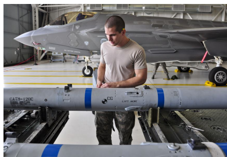
AMRAAM A1C Zoller makes an AIM-120 advanced medium-range air-to-air missile safe before loading it onto an F-35A Lightning II.
