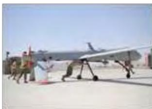
An MQ-1 Predator being pushed to a hangar for maintenance
