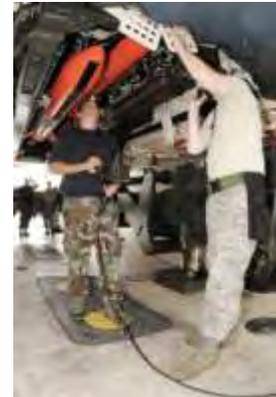
**An Airman inspects the rotary launch assembly as it is being lifted into a B-2**
