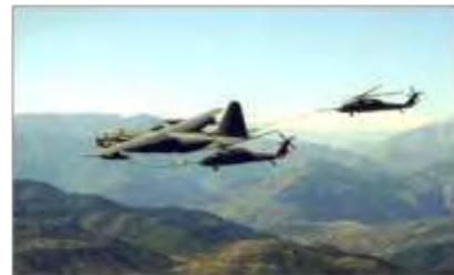
**HC-130P provides critical capabilities to joint and coalition forces to include aeromedical evacuation, insertion of Guardian Angel pararescue forces and inflight helicopter aerial refueling to extend the range of the HH-60G**
