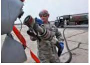
Fueling an A-10C with a biomass-derived fuel blend
