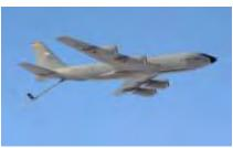
A KC-135 Stratotanker with its boom fully extended for refueling
