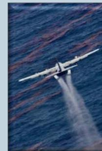
C-130 drops an oil-dispersing chemical as part of the Deepwater Horizon Response.
